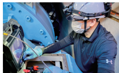
Using an endoscope to examine the inside of equipment
